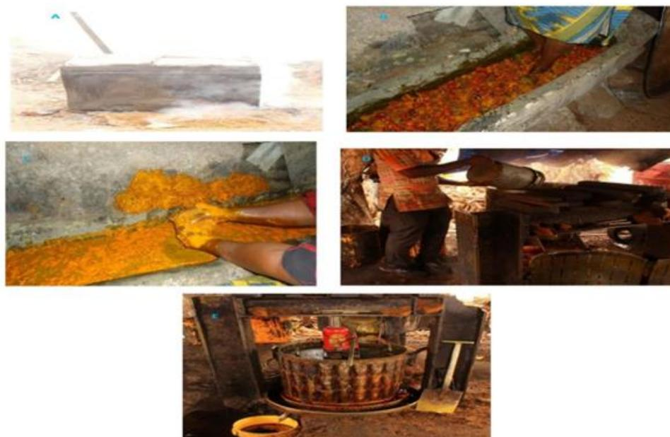
Figure 3. Palm oil processing:(A) boiling of fruit (B), traditional fruit digestion by mashing with the feet (C),traditional oil filtration (D), semi-mechanized fruit digestion (E), and semi-mechanized oil separation
