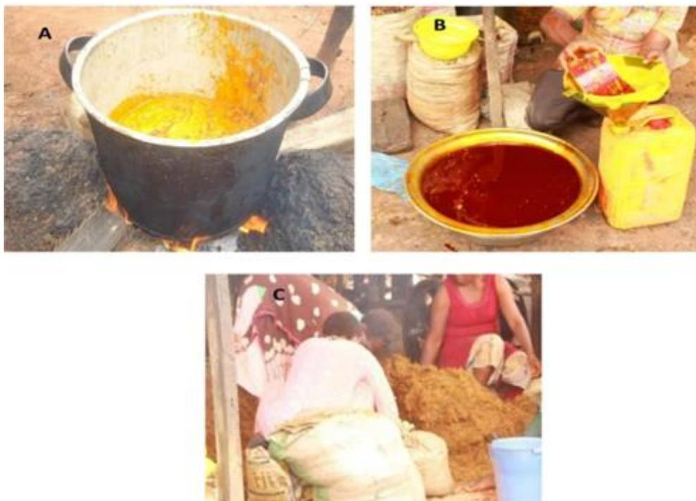
Figure 4. Showing last phase of processing: (A) Oil clarification (B) Oil filtration (C), Separation of kernel from the fibre at Umuahia North Abia State Nigeria
